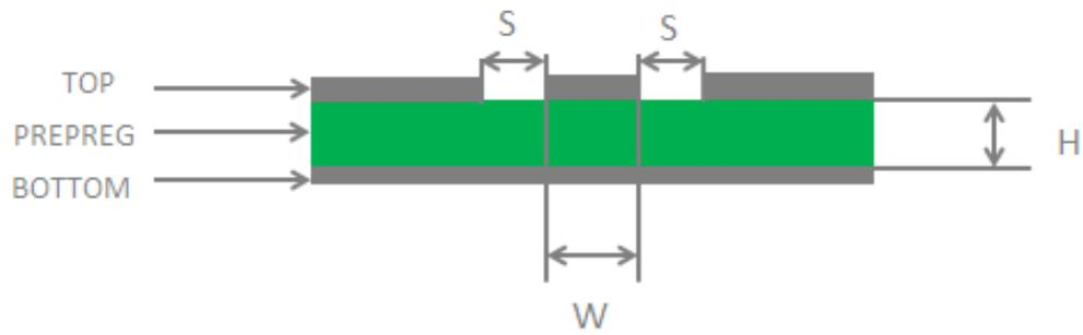
Figure 32: Coplanar Waveguide Design on a 2-layer PCB
