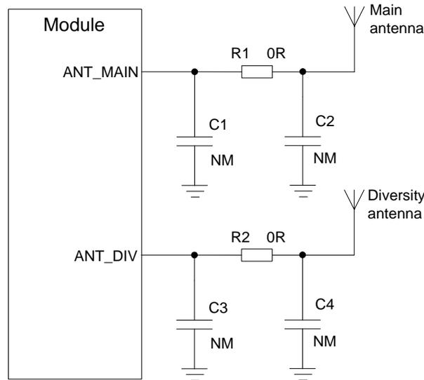
Figure 30: Reference Circuit of RF Antenna Interface
