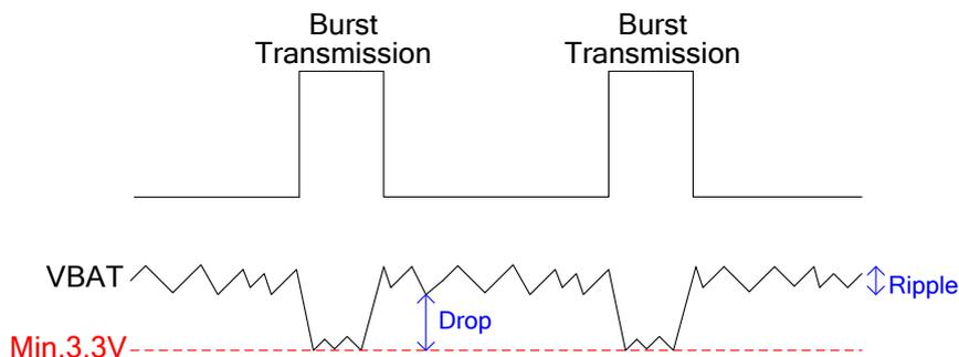
**Figure 7: Power Supply Limits during Burst Transmission**
