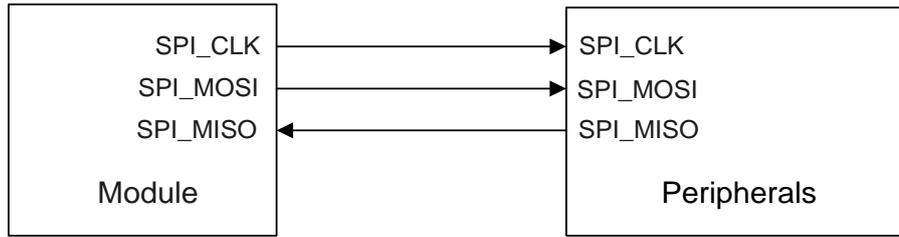
Figure 25: Reference Circuit of SPI Interface with Peripherals
