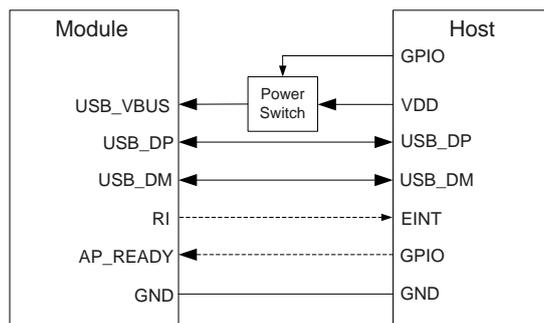
**Figure 6: Sleep Mode Application without Suspend Function**
