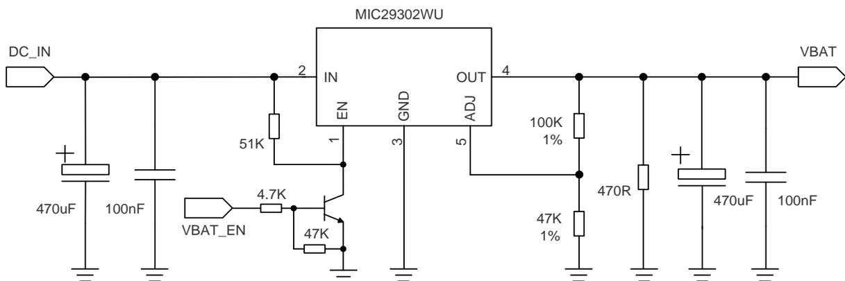
Figure 9: Reference Circuit of Power Supply
