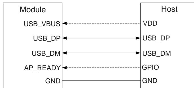
**Figure 4: Sleep Mode Application with USB Remote Wakeup**
