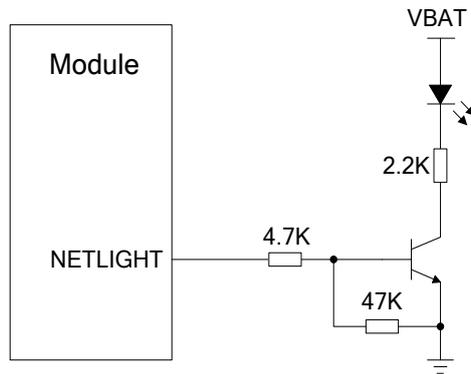
Figure 26: Reference Circuit of Network Status Indicator
