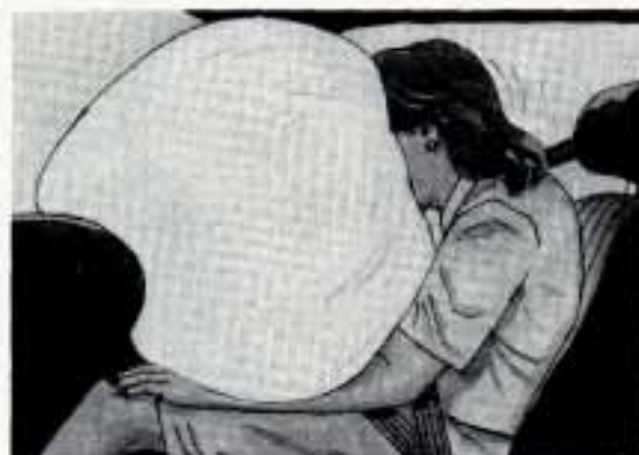
The right-front passenger's air bag is located in the instrument panel on the passenger's side.
