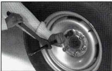
With the DOWN side facing you, use the ratchet and socket to loosen all the wheel nuts. Don't remove them yet.
