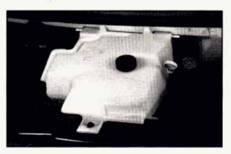
When your engine is cold, the coolant level should be at FULL COLD, or a little higher.
