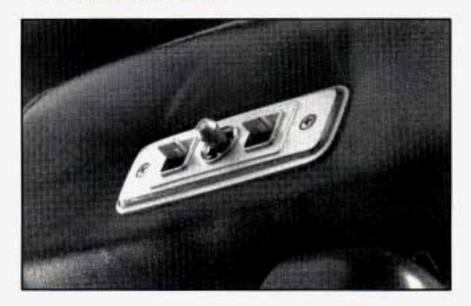
If your vehicle has a power seat on the driver's or passenger's side, you can adjust it with this switch at the front center cushion of the seat.
