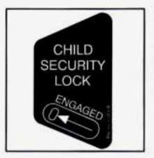
Move the button to the left to engage the security feature. Move the button to the right to return the door locks to normal operation.
