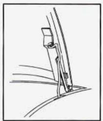
Lift the hood, release the hood prop from its retainer and put the hood prop into the slot in the hood hinge. The underhood lamp will automatically come on and stay on until the hood is closed.
