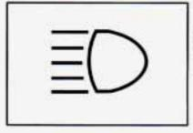
When the high beams are on, this light on the instrument panel also will be on.
