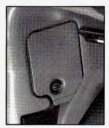
The fuse block access door is on the driver's side of the instrument panel above the hood release lever.
