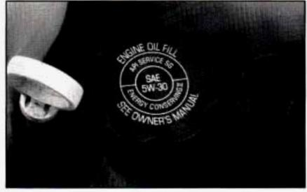
The engine oil filler cap is located between the coolant recovery tank and the air cleaner. Be sure to fill it enough to put the level somewhere in the proper operating range. Push the dipstick all the way back in when you're through.
