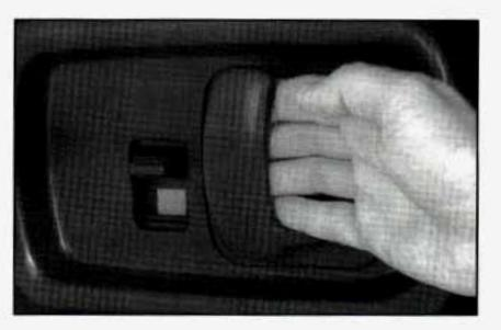
To open the "60" (front) portion of a 60/40 door from the inside, pull the handle toward you and push open the door.
