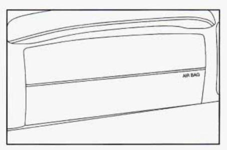
If it says AIR BAG on the middle part of the steering wheel and AIR BAG on the instrument panel in front of the right front passenger's seat, your vehicle has two air bags -- one air bag for the driver and another air bag for the right front passenger.
