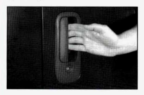
To open the "60" (front) portion of a 60/40 door from the outside, pull up on the handle and pull the handle toward you.
