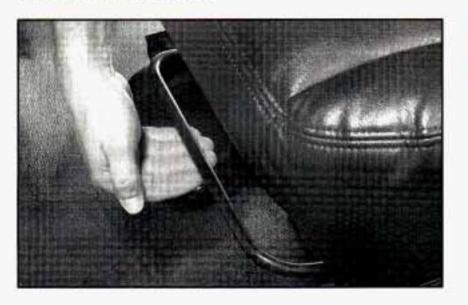
The bucket seats can be adjusted forward or rearward with the lever at the front of the seat.
