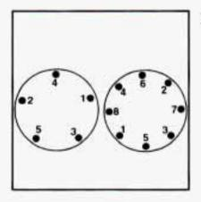
Tighten the nuts firmly in a crisscross sequence as shown. Rotate the wheel wrench to the right.
