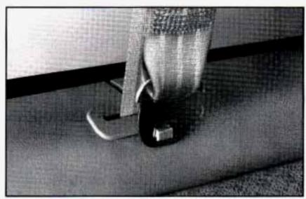
10. For the first rear seat, stow the safety belt latch by attaching the fastener strip on the safety belt latch to the trim just inside the side door. There is also a fastener strip provided for stowing the safety belt latch for a four-passenger bench seat, if equipped.
