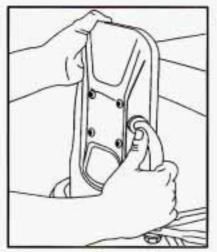
To adjust the mirrors when towing a trailer, rotate the mirror by pushing the mirror head toward the front of the vehicle.
