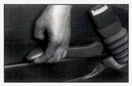
To adjust the seatback, lift the front of this lever, which is located at the inner edge of the seat cushion.
