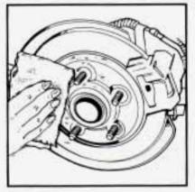
Remove any rust or dirt from the wheel bolts, mounting surfaces and spare wheel.
