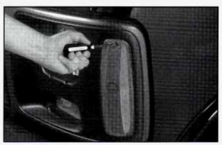
Remove the screw from the top of the lens.
