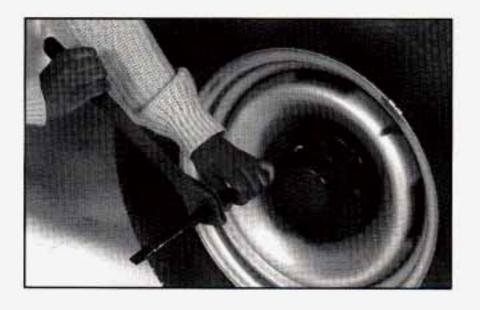
You will need to take off the wheel nut caps to reach your wheel nuts. When using the ratchet and socket, make sure the DOWN side faces you.
