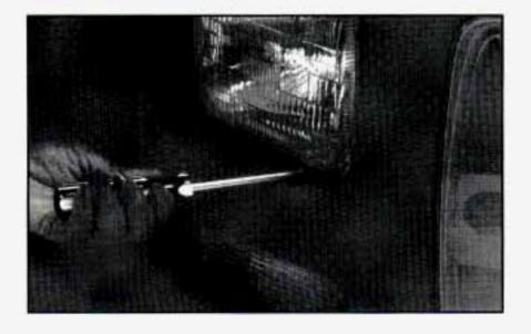
Remove the four screws from the headlamp retainer. Pull the retainer out and set it aside.
