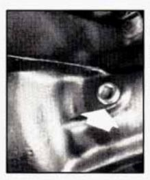
If the level is below the bottom of the filler plug hole, you'll need to add some lubricant. Add enough lubricant to raise the level to the bottom of the filler plug hole.
