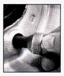
Replace the wheel nuts with the rounded end of the nuts toward the wheel. Tighten each wheel nut by hand until the wheel is held against the hub.
