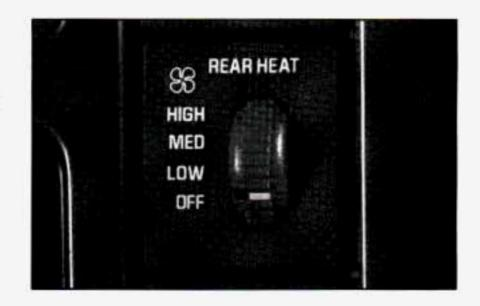
To increase and decrease the flow of heated air to the rear floor vents, move the switch marked REAR HEAT to the blower speed you want.
