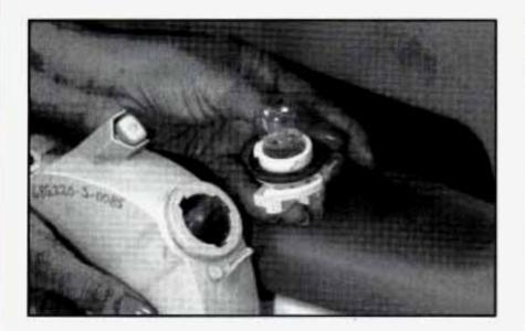
Squeeze the tab on the side of the bulb assembly while turning it to the left. Remove the bulb assembly from the back of the lens and replace the bulb.
