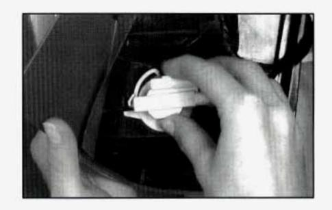
Squeeze the tab on the side of the sockets while turning them to the left to remove.
