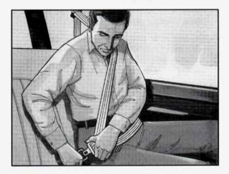
Pick up the latch plate and pull the belt across you. Don't let it get twisted. Push the latch plate into the buckle until it clicks.
