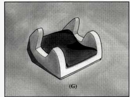
A booster seat (F, G) is designed for children who are about 40 to 60 lbs. (18 to 27 kg) and about four to eight years of age. It's designed to improve the fit of the vehicle's safety belt system. Booster seats with shields use lap-only belts; however, booster seats without shields use lap-shoulder belts. Booster seats can also help a child to see out the window.
