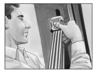
To move the height adjuster down, push in at the word PRESS and move the height adjuster to the desired position. You can move the adjuster up just by pushing up on the shoulder belt guide. After you move the adjuster to where you want it, try to move it down without pushing in to make sure it has locked into position.
