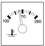
This gage shows the engine coolant temperature.
