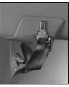
Then, hang the latch plate end of the belt on the hook at the top of the retractor cover, out of the way.
