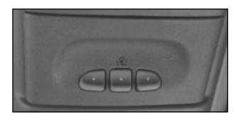
This transmitter allows you to consolidate the functions of up to three individual hand-held transmitters. It will operate garage doors and gates, or with the accessory package, other devices controlled by radio frequency such as home/office lighting and security systems.
