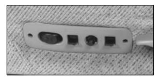
If your vehicle has a power seat on the driver's or passenger's side, you can adjust it with these controls at the outside edge of the seat. The switch is located on the side of the seat, next to the door.
