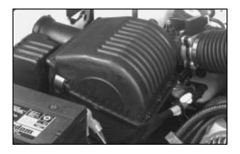
Your air cleaner is located between the battery and coolant recovery tank.
