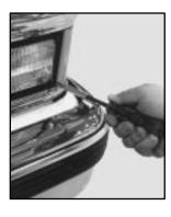
Remove the four screws and take out the parking/turn signal lamp assembly.
