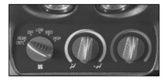
To adjust the airflow speed, turn the fan control knob on the left side of the control panel to the desired blower setting.
