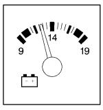
When your engine is not running, but the ignition is in the RUN position, this gage shows your battery's state of charge in DC volts.
