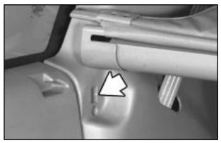
To put the shade in the vehicle, first make sure the shade slot in the holder faces rearward with the round surface facing down. Then, hold the shade at an angle and place the shade holder tab into the slot in the passenger's side trim panel. Move the other end of the shade forward and hold it next to the driver's side trim panel slot.
