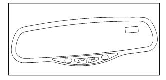
The mirror also includes a display in the upper right corner of the mirror face. This can be used as a compass or to indicate outside air temperature.
