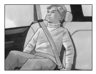
Buckle, position and release the safety belt as described in "Rear Seat Outside Passenger Positions" earlier in this section. Make sure that the shoulder belt crosses the shoulder.
