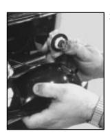
3. Pull the socket out of the lamp assembly.
