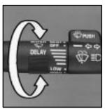
You control the windshield wipers by turning the knob with the wiper symbol on it.
