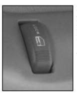
Press the side of the power door lock switch marked LOCK on either front door to lock all the doors at once. Press the ribbed side of the switch to unlock all the doors at once.
