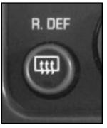
To turn on the rear window defogger, press this button next to the fan control knob. The rear window defogger will only work if the ignition switch is turned to RUN. For best results, first clear the window of as much snow or ice as possible.
