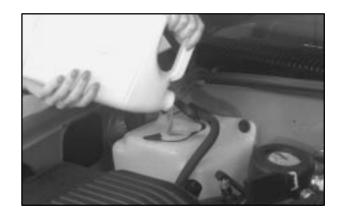
You can be burned if you spill coolant on hot engine parts. Coolant contains ethylene glycol and it will burn if the engine parts are hot enough. Don't spill coolant on a hot engine.
