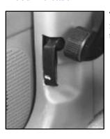
To open the hood, first pull the handle inside the vehicle.
