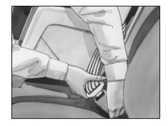
3. Buckle the belt. Make sure the release button is positioned so you would be able to unbuckle the safety belt quickly if you ever had to.
