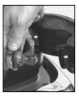
Squeeze the tab on the side of the lamp socket while turning the socket counterclockwise.
