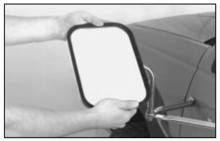
2. Rotate the mirror head, so that the mirror surface faces the rear of the vehicle.
