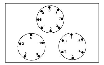
10. Tighten the nuts firmly in a crisscross sequence as shown. Rotate the wheel wrench clockwise.
