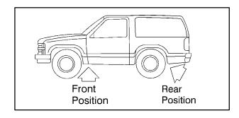
3. Position the jack under the vehicle. If the flat tire is on the front of the vehicle, position the jack on the frame behind the flat tire. If the flat tire is on the rear of the vehicle, position the jack on the axle near the flat tire between the spring and the shock absorber.
