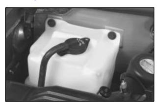
The coolant recovery tank is located on the passenger's side at the rear corner of the engine compartment.
