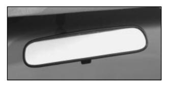
Pull the tab under the mirror to reduce glare from headlamps behind you after dark. Push the tab forward for normal daytime operation.
