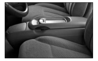
To open it, lift the latch handle and swing the door open.
