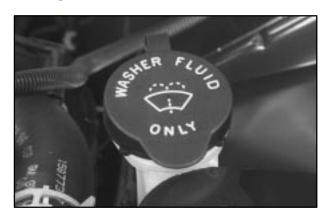
Open the cap labeled WASHER FLUID ONLY. Add washer fluid until the tank is full.
