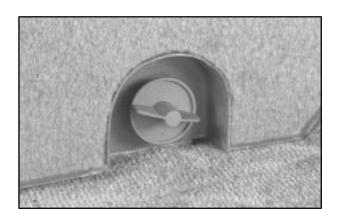
To open the jack cover on four-door utility models, turn the wing nut counterclockwise and take the cover off.
