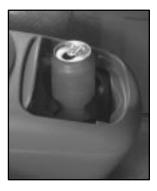
Your vehicle may have a removable cupholder at the front of the console. To remove the cupholder, pull the front of the cupholder toward you and lift up.
