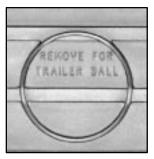
If you will be using the bumper to tow a trailer, you must remove the center cutout circle to install the trailer ball. You must also remove both outer cutouts to attach the trailer safety chains.
