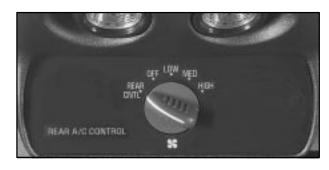
To operate the rear system using the front control, just turn the knob to the blower position you want. To use the rear control, first turn the front control knob to REAR CNTL.
