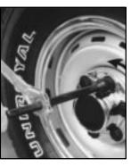
If your vehicle has wheel nut caps, use the wheel wrench and ratchet to remove them. Turn the wheel wrench counterclockwise, with DOWN facing you, to remove the wheel nut caps. Then take off the hub cap.
