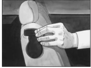
Remove the guide from its storage clip on the side of the seatback.
