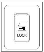
On the passenger side of the rear cargo door or tailgate, there is a power lock switch which can be used to lock or unlock all of the doors.
