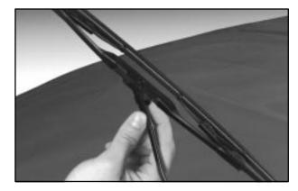
Windshield wiper blades should be inspected at least twice a year for wear or cracking. See "Wiper Blade Check" in Section 7 of this manual under Part B "Owner Checks and Services" for more information.
