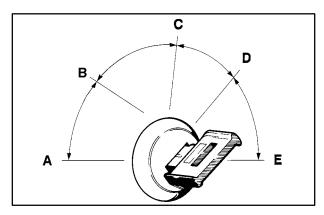
**ACCESSORY** (A): This position lets you use things like the radio and the windshield wipers when the engine is off. Push in the key and turn it toward you. Your steering wheel will remain locked, just as it was before you inserted the key.
