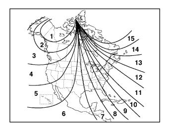
4. Press the COMP button on the bottom of the mirror until the new zone number appears in the display. After you stop pressing the button in, the display will show a compass direction within a few seconds.
