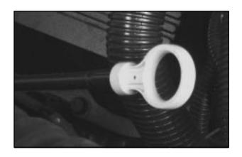
The engine oil dipstick has a yellow ring handle and is located on the passenger's side of the engine.
