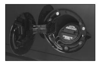
The fuel cap is located behind a hinged door on the driver's side of your vehicle.
