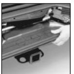
To remove the pad, lift the edge of the pad from the rear of the bumper and swing it forward. When the pad releases from the bumper holes, lift the pad off.
