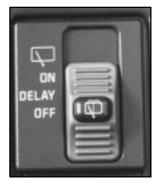
The rear window wiper and washer switch is on your instrument panel, to the right of the gage cluster.
