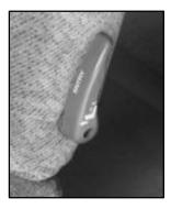
To operate the seat, pull forward on the top of the lever located at the side of the seatback, and tilt the seatback forward toward the front of the vehicle.
