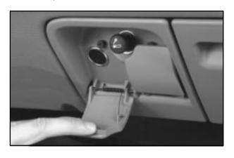
Two auxiliary power outlets are located near the cigarette lighter. Use these outlets to power mobile telephones or other devices designed to operate with vehicle electrical systems.
