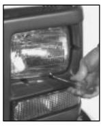
1. Remove the four screws from the headlamp retainer.
