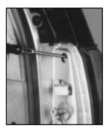
3. Remove the two rear lamp assembly screws inside the fender and pull out the lamp assembly. You may want to use a magnetic screwdriver when removing the screws.
