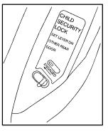
With this feature, you can lock the rear side doors so they can't be opened from the inside by passengers.
