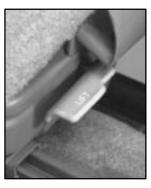
There is a foot-operated release lever for rear seat passengers to use when getting out of the third seat.
