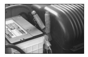
6. Connect the red positive (+) cable to the positive (+) terminal of the vehicle with the dead battery.
