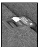
On Suburban models, to create a load floor, release the panels from the seatback by pushing rearward on the latch and fold them out to cover the rear seat footwell.
