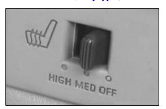
The control for the driver's side heated seat is located on the left side of the seat. The control for the right front passenger is located on the right side of the passenger's seat. Move the switch forward to MED or HIGH temperature to turn on the heating elements in the seat. The right front passenger's safety belt must be buckled before the heating elements in that seat will operate. To turn the heated seats off, move the switch rearward to OFF.
