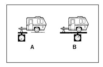
If you're using a weight-carrying hitch, the trailer tongue (A) should weigh 10 percent of the total loaded trailer weight (B). If you're using a weight-distributing hitch, the trailer tongue (A) should weigh 12 percent of the total loaded trailer weight (B).
