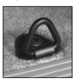
There are cargo tie downs in the rear cargo area that allow you to strap cargo in and keep it from moving inside the vehicle.
