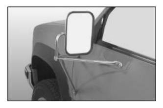
If your vehicle is equipped with the camper type mirrors, they can be adjusted so you can have a clear view of objects behind you.
