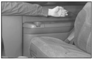
When you release the seat cushion, the seatback is automatically released. Pull the loop on the seatback forward and fold the seatback onto the seat cushion.
