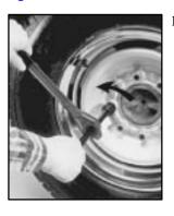
1. Use the ratchet and wheel wrench to loosen all the wheel nuts. Turn the wheel wrench counterclockwise, with DOWN facing you, to loosen the wheel nuts. Don't remove the wheel nuts yet.
