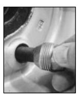
7. Replace the wheel nuts with the rounded end of the nuts toward the wheel. Tighten each wheel nut by hand using the wheel wrench until the wheel is held against the hub.
