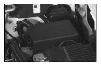
The underhood fuse/relay center is located in the rear of the engine compartment near the brake fluid reservoir. Move the retainer clips for the cover to access the fuse block.
