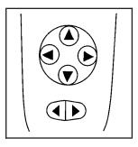
The controls for the outside power mirrors, are located on the driver's door armrest.
