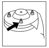
The remote negative (–) ground terminal, marked GND (–), is located behind the engine coolant surge tank.
