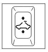
Your vehicle may be equipped with a power sunroof. The switch that operates it is located on the headliner.
