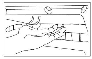
Open the passenger compartment air filter door by reaching through the opening in the back of the glove box and raising the tab until the door can be opened downward.
