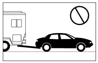
Notice: Towing your vehicle from the rear could damage it. Also, repairs would not be covered by the warranty. Never have your vehicle towed from the rear.
