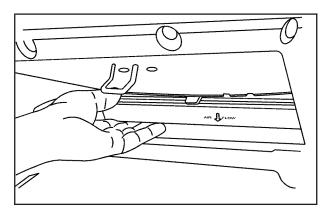
4. Remove the filter by sliding it out of the housing.
