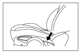
Your vehicle has reclining seatbacks. The lever is located on the outboard side of the seats. Lift the lever to release the seatback. Move the seatback to where you want it and release the lever to lock the seatback in place. Press rearward on the seatback to be sure it is locked into place.
