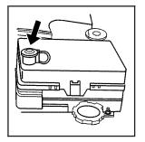
The remote positive terminal is located under a red tethered cap on the engine compartment fuse block. Lift the cap to access the terminal.
