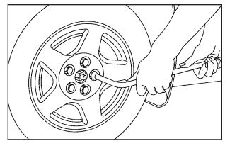
If your vehicle is equipped with plastic wheel covers, use the wheel wrench to loosen the plastic wheel nut caps.
