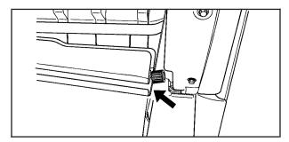
Tilt the glove box door down by squeezing on each side of the glove box until the door can be lowered from its track. Lower the glove box door.
