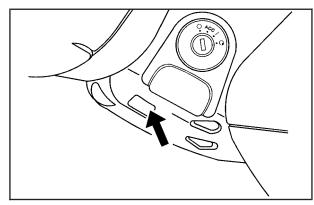
2. Using a tool, pry off the cover from the bottom of the steering column.
