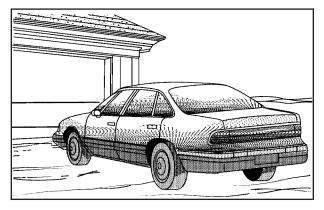
4. Turn on the low-beam headlamps and place a piece of cardboard or equivalent in front of the headlamp not being aimed. This should allow only the beam of light from the headlamp being aimed to be seen on the flat surface.
