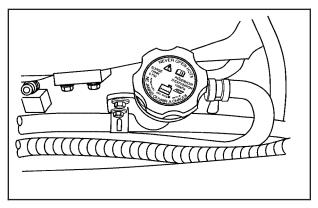
The intercooler system fill neck is located in the front of the engine compartment, near the center of the vehicle. See *Engine Compartment Overview on page 5-12* for more information on location.
