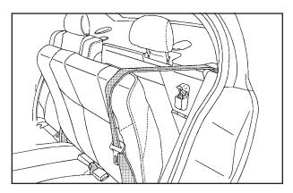
Once the handle is pulled, the seatback can be pushed open through the trunk, or pulled open from the inside of the vehicle. To raise the rear seatback, lift it up and push rearward until you hear a click. Push and pull on the seatback to be sure it is locked into place.
