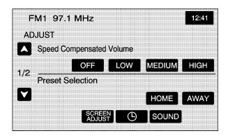
**Automatic Volume Control (AVC):** With AVC, the audio system will adjust automatically to make up for road and wind noise as you drive, by increasing the volume as vehicle speed increases.
