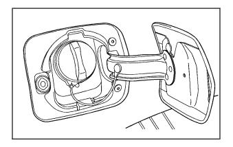
The tethered fuel cap is located behind a hinged fuel door on the passenger side of the vehicle. If the vehicle has E85 fuel capability, the fuel cap will be yellow and state that E85 or gasoline can be used. See *Fuel E85 (85% Ethanol) on page 6-8*.
