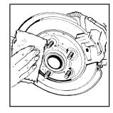
Remove any rust or dirt from the wheel bolts, mounting surfaces, and wheel.
