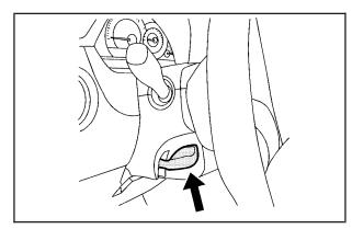
The adjustment lever is located on the left side of the steering column.
