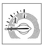
The vehicle has an engine coolant temperature gage. With the ignition turned to ON/RUN, this gage shows the engine coolant temperature.
