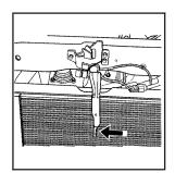
2. Then go to the front of the vehicle and push the secondary hood release lever to the left. It is located under the front center of the grille.
