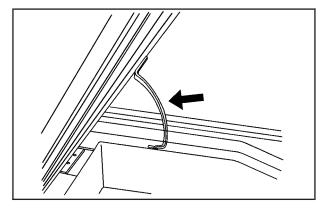
There is a rod that hooks into place to prop open the lid. Push the rod towards the lid to unhook it and lower the lid.
