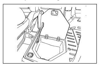
The vehicle may have two storage bins located in the rear of the vehicle. Pull up on the handles to open and lift the lid. Use the key to lock/unlock the bins.
