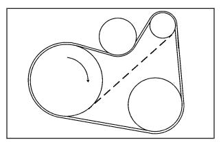
Dotted line shows routing for vehicles without air conditioning.
