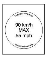
16. If the flat tire was able to inflate to the recommended inflation pressure, remove the maximum speed label from the sealant canister and place it in a highly visible location. The label is a reminder not to exceed 55 mph (90 km/h) until the damaged tire is repaired or replaced.
