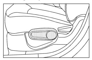
If your vehicle has this feature, the driver's seat height adjuster is located on the outboard side of the seat.
