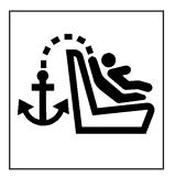
To assist you in locating the top tether anchors, this symbol is located next to each top tether anchor.
