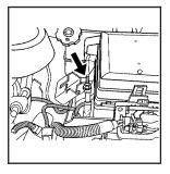
Locate the remote positive terminal which is located under a red tethered cap on the engine compartment fuse block. Remove the cap to access the terminal.
