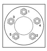
11. Tighten the wheel nuts firmly in a crisscross sequence as shown.
