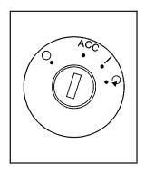
The ignition switch has four different positions.
