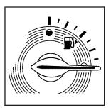
The fuel gage indicates about how much fuel is left in the fuel tank.
