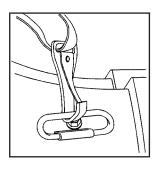
9. Attach the strap to the cargo tie-downs in the rear of the vehicle.
