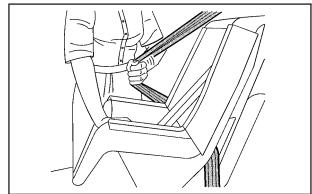
4. Pull the rest of the shoulder belt all the way out of the retractor to set the lock.
