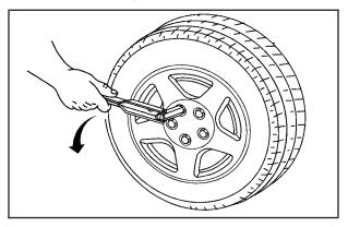
Using the wheel wrench, loosen all the wheel nuts on the rear tire. Do not remove them yet.
