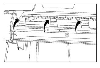
3. Pull the three tabs of the filter access door down and open the access door downward.
