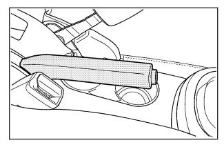
The parking brake lever is located between the front seats.
