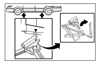
Position the jack on the front position and raise the jack lift head to fit over the car flange under the down arrow markings on the rocker panel.
