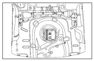
Turn the retainer clockwise and remove the tire sealant and compressor kit.
