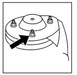
Locate the remote negative (–) ground terminal, marked GND (–), which is located at the front of the engine compartment on the driver side of the vehicle.
