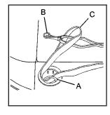
Route the loop end of the strap (C) through one of the cargo tie-downs (A) located in the rear of the vehicle.
