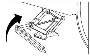
Raise the vehicle by turning the jack handle clockwise. Raise the vehicle far enough off the ground so there is enough room for the compact spare tire to fit underneath the wheel well.
