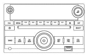
Radio with CD (MP3) and USB Port shown, Radio with CD (MP3) similar
