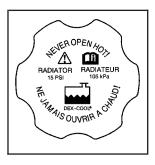
Remove the pressure cap when the cooling system, including the pressure cap and upper radiator hose, is no longer hot.
