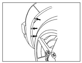
Remove the fasteners located on the wheel liner. To access the headlamp and the turn signal/parking lamp bulbs.
