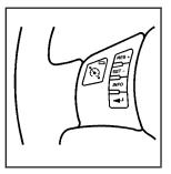
The cruise control buttons are located on the left side of the steering wheel.
