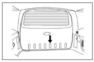
Remove the trim plug, located on the inside of the liftgate near the center.
