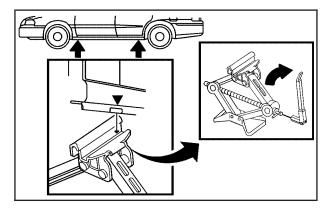
Position the jack on the rear position and raise the jack lift head to fit over the car flange under the down arrow markings on the rocker panel.
