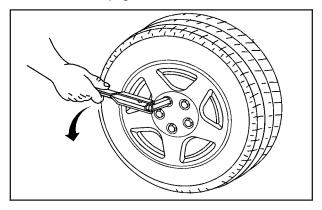
Using the wheel wrench, loosen all the wheel nuts. Do not remove them yet.
