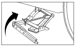
4. Raise the vehicle by turning the jack handle clockwise. Raise the vehicle far enough off the ground so there is enough room for the compact spare tire to fit underneath the wheel well.
