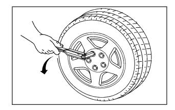
2. Using the wheel wrench, loosen all the wheel nuts on the front flat tire. Do not remove them yet.
