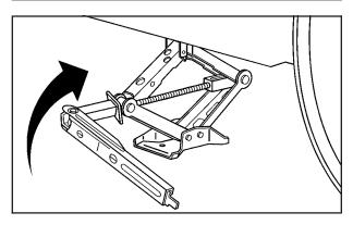
Raise the vehicle by turning the jack handle clockwise. Raise the vehicle far enough off the ground so there is enough room for the tire.
