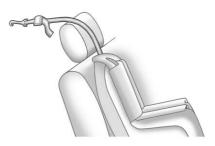
If the position you are using has a fixed headrest or head restraint and you are using a single tether, route the tether over the headrest or head restraint.
