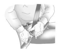
To unlatch the belt, push the button on the buckle. For outboard seating positions, slide the latch plate up the safety belt webbing when the safety belt is not in use. The latch plate should rest on the stitching on the safety belt, near the guide loop.
