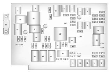
**Engine Compartment Fuse Block**
