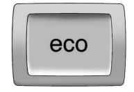
Press the "eco" (economy) button by the shift lever to turn this feature on or off. The "eco" light in the instrument cluster will come on when engaged. See Fuel Economy Light on page 4-22. For vehicles with a Driver Information Center (DIC) an "ECO Mode On" message displays. See Fuel System Messages on page 4-30 for more information.
