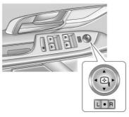
Controls for the outside power mirrors are located on the driver door.
