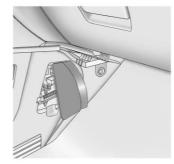
The instrument panel fuse block is located on the passenger side panel of the center console. To access the fuses, open the fuse panel door from the passenger side by pulling it out.
