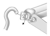
8. Fit the jack handle extension onto the jack by sliding the hook through the end of the jack.
