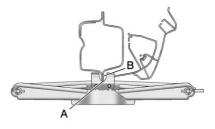
Place the jack notch (A) under the frame rail seam (B).
