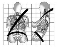
Sit up straight and always keep your feet on the floor in front of you. The lap part of the belt should be worn low and snug on the hips, just touching the thighs. In a crash, this applies force to the strong pelvic bones and you would be less likely to slide under the lap belt. If you slid under it, the belt would apply force on your abdomen. This could cause serious or even fatal injuries. The
