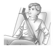
Buckle, position, and release the safety belt as described previously in this section. Make sure that the shoulder belt crosses the shoulder. To remove and store the comfort guide, squeeze the belt edges together so that the safety belt can be removed from the guide. Slide the guide back into its storage pocket located on the side of the seatback.
