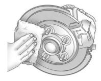
Remove any rust or dirt from the wheel bolts, mounting surfaces, and spare wheel. 15. Place the compact spare tire on the wheel-mounting surface.
