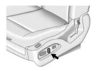
On vehicles with power reclining seatbacks, the switch is located on the outboard side of the seat. See *Power Seat Adjustment on* page 2-3 for more information.
