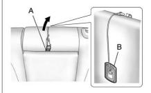
Stow the rear seat center armrest. Attach the retaining strap to the armrest loop (A) and to the center top tether anchor on the seatback (B). Make sure the retaining strap's clips are firmly attached.
