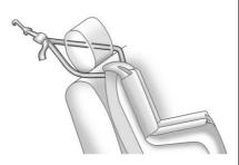
If the position you are using has a fixed headrest or head restraint and you are using a dual tether, route the tether around the headrest or head restraint.
