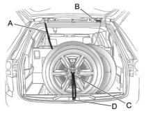
Pull the cable (A) through the door striker (D) then the center of the wheel (C).
