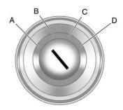
The ignition switch has four different positions.
