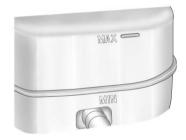
The fluid level should be above MIN. If it is not, have the brake hydraulic system checked to see if there is a leak.
