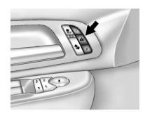
On vehicles with the memory feature, the controls on the driver door are used to program and recall memory settings for the driver seat, outside mirrors, and the adjustable throttle and brake pedals.
