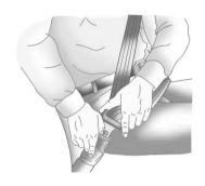
To unlatch the belt, push the button on the buckle. The belt should return to its stowed position.
