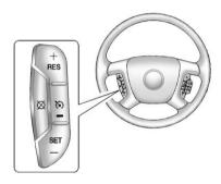
Press to turn the system on or off. The indicator light is on when cruise control is on and turns off when cruise control is off.
