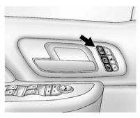
Heated and Cooled Seat Buttons Shown, Heated Seat Buttons Similar
