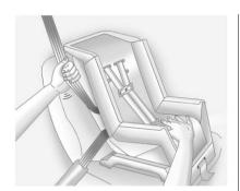
6. To tighten the belt, push down on the child restraint, pull the shoulder portion of the belt to tighten the lap portion of the belt, and feed the shoulder belt back into the retractor. When installing a forward-facing child restraint, it may be helpful to use your knee to push down on the child restraint as you tighten the belt.
