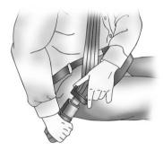
Push the latch plate into the buckle until it clicks. If you find that the latch plate will not go fully into the buckle, see if you are using the correct buckle.
