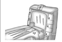
Fold the seatback forward until it is flat. If necessary, move the front seats forward slightly to allow the seatback to fold completely. 4. Repeat the procedure for the other seatback, if desired.
