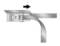
4. Tighten all straps by pulling on the free end of each strap.
