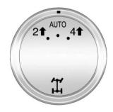
The transfer case knob is located to the left of the instrument panel cluster.
