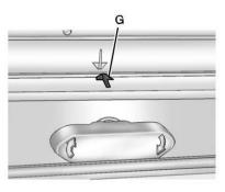
Be sure to align the rear glass side-to-side using the glass alignment arrows (G).
