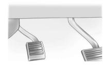
Set the parking brake by holding the regular brake pedal down, then pushing down the parking brake pedal.
