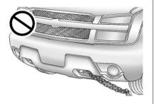
Notice: Never use recovery hooks to tow the vehicle. Your vehicle could be damaged and it would not be covered by warranty.
