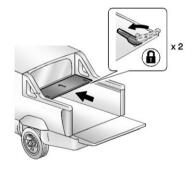
The driver side cargo cover panel latch must lock in place before the passenger side latch can be locked. If this procedure
