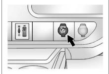
This vehicle also has a USB port on the instrument panel.
