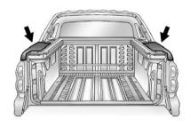
There are top-box storage units on both sides of the rear cargo area. The passenger side contains the tire changing tools. To lock or unlock, use the key then press the key cylinder to open.
