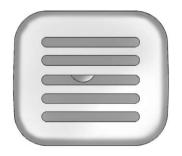
There is also an interior temperature sensor located next to the steering wheel that measures the temperature of the air inside your vehicle.
