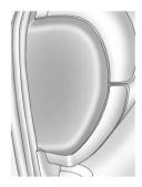
The instrument panel fuse block access door is located on the driver side edge of the instrument panel.
