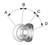
The ignition switch has four different positions.
