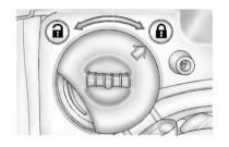
Once both glass lock knobs are in the locked position, the rear glass is securely stored.
