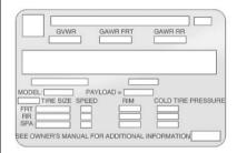
A vehicle specific Certification/ Tire label is attached to the rear edge of the driver door. The label shows the size of your vehicle's original tires and the inflation pressures needed to obtain the gross weight capacity of your vehicle. This is called Gross Vehicle Weight Rating (GVWR). The GVWR includes the weight of the vehicle, all occupants, fuel and cargo.
