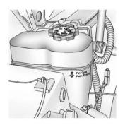
The coolant surge tank is located in the engine compartment on the passenger side of the vehicle. See *Engine Compartment Overview on page 10-5* for more information on location.
