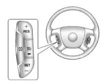
(On/Off): Press to turn the system on or off. The indicator light is on when cruise control is on and turns off when cruise control is off.
