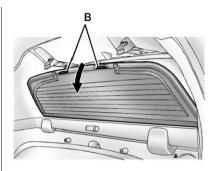
4. With the rear glass tilted toward vou. lift it out from the lower window frame channel. Use the grab handles (B) to assist you in removing the rear glass.
