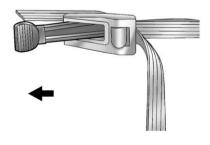
Close both cross locks at the center of the strap system to tightly secure.
