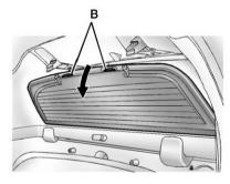
4. With the rear glass tilted at an angle, place the bottom edge in the lower channel of the window frame.
