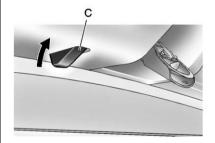
3. While holding the rear glass in place, press the glass-catch release button (C) and pull the top of the rear glass toward you using the grab handles (B) located at the top of the rear glass.
