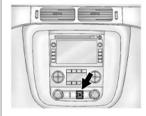
The vehicle may have power assist steps. To enable or disable the power assist steps push ...
