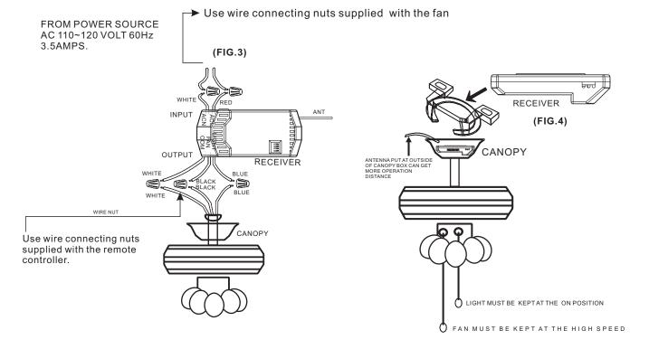
If other fans or supply wires are different color, have this unit installed by qualified licensed electrician.
