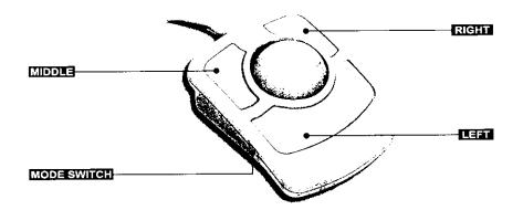
If change to Left Hand User, please turn off the computer first, and switch the Mode Switch (on the left side of the trackball) to PC mode, and use the attached Driver to re-locate the button positions. The positions will be:
