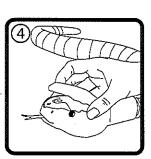
4) To insert batteries into the snake, lift off the upper head section revealing the panel below.
