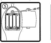
5) Un-screw the battery cover using a Philips head Screwdriver and remove. Insert 4x AAA batteries, into the head section, following the polarities indicated on the battery compartment.
