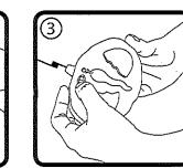
2) Insert one 9V (6LR61) 3) On the controller slide the battery, following the polarities switch to the ON position. indicated on the battery compartment. Re-screw the back panel removed in step one.
