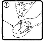
1) To insert batteries into the controller, unscrew and remove the rear panel using a Philips screwdriver.
