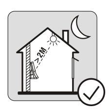
When installing outdoors, direct sunlight equipment, oblique sunlight equipment or direct sunlight equipment through window are prohibited When installing indoors, make sure that the place must be installed away from windows / doors / lamp more than 2 meters away equipment
