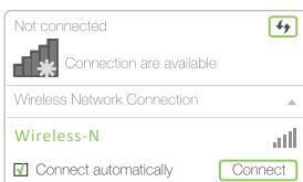
Disconnect your Ethernet (wired) connection from your computer. Click the Wi-Fi icon on the taskbar and connect to the Repeater's network (e.g. **Wireless-N**).
