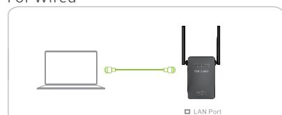
Disable the Wi-Fi on your computer. Connect your computer to the Repeater via an Ethernet cable.
