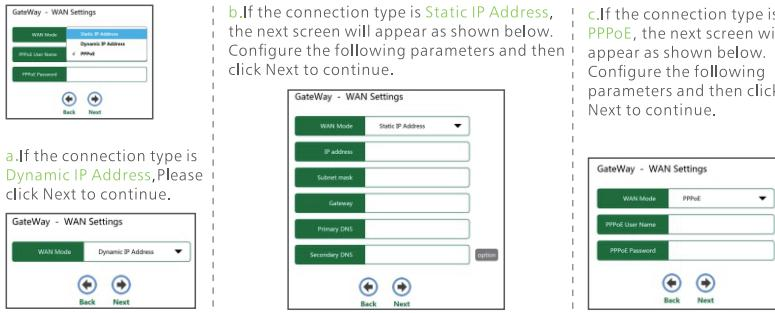
**IP Address** - This is the WAN IP address as seen by external users on the Internet (including your ISP). Enter the IP address into the field.
