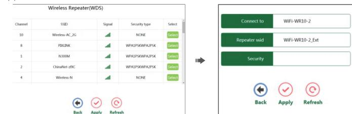
Select the SSID of the target network and insert Repeater SSID and the key of your network. the default Repeater SSID is set to be **xxxx\_Ext** (xxxx indicates The Main Router's wireless network name). Then click **Apply** to complete setup.
