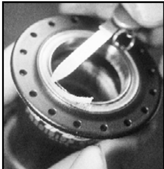
Figure 12 - remove snap ring
