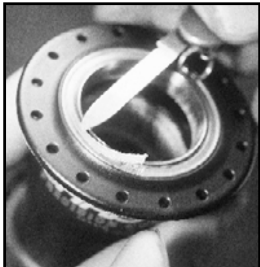
Figure 53 - remove snap ring
