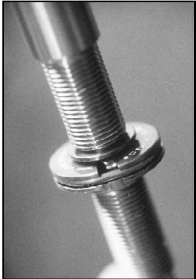
Figure 17 - function of the split ring
