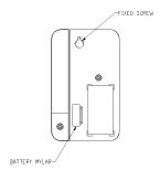
If there is no battery inside the detector or need to replace a new battery please insert the battery in 45° angle as below figure
