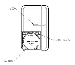
The Door/Window contact detector consists of two parts; a Detector and a Magnet. They are designed to be fitted to doors or windows with the Magnet mounted on the opening part and the Detector mounted on the fixed frame. Opening the protected door/window will remove the magnetic field, trigger the Detector and generate an alarm condition, (if the system is armed).
