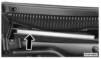
3. Install the new filter with arrows pointing in the direction of airflow, which is toward the rear of the vehicle (text and arrows on the filter will indicate this).
