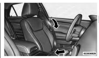
Pulling Out the Lap/Shoulder Belt Latch Plate
