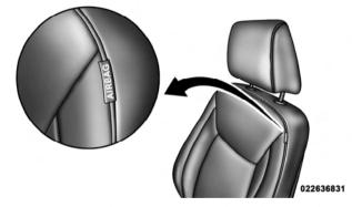
Supplemental Seat-Mounted Side Airbag Label When the airbag deploys, it opens the seam between the front and side of the seat's trim cover. Each airbag
