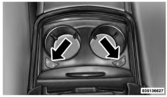
Heated And Cooled Cupholder Switches
