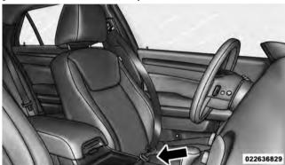
**Inserting Latch Plate Into Buckle**
