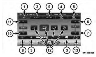
Uconnect Touch™ System 8.4 Automatic Temperature Controls — Soft-keys
