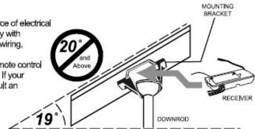
CAUTION: FOR MOUNTING RECEIVER, CEILING ANGLE SHALL NOT EXCEED 19 DEGREES RECEIVER MODEL: CFR-3D
