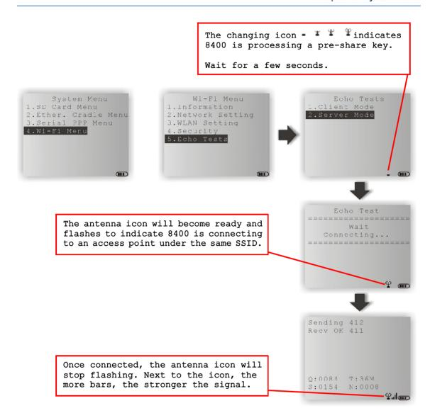
Note: If you are programming in C or BASIC, be aware that these icons will appear on the device screen after NetInit() or START TCPIP() is called. (WPA must be enabled first!)
