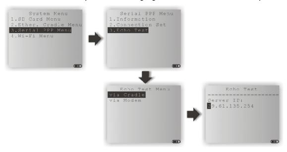
Note: Enter the IP address of a server with which a PPP connection is desired. Then, it will try to connect to the server. After the PPP connection is established properly, run the utility "EchoTest.exe" on your computer (TCP/IP – Server), and then, start this test on your mobile computer.
