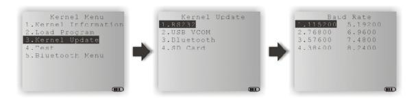
Note: CipherLab software, including download utilities, supports the following baud rate options: 115200/57600/38400/19200/9600 bps.
