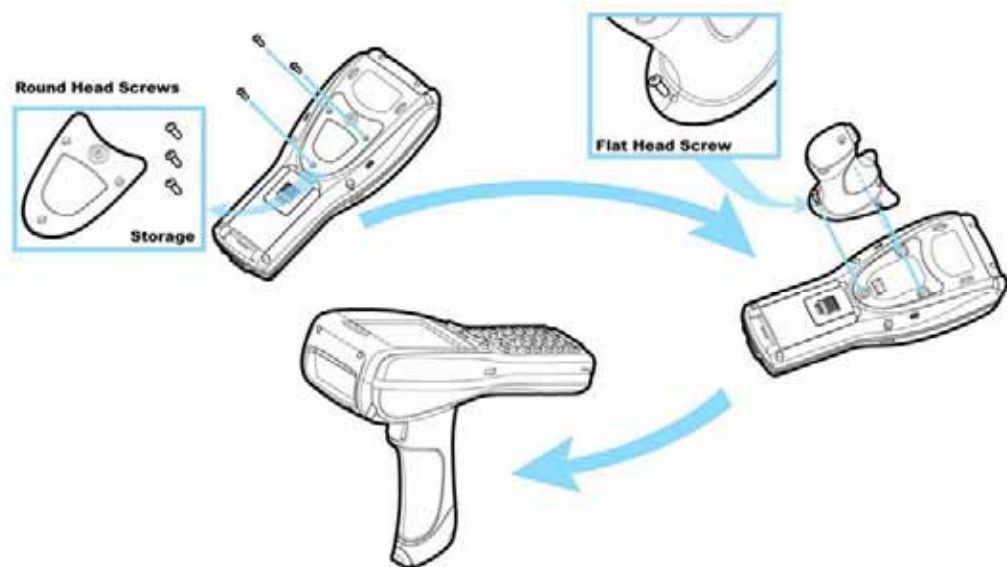
Figure 8: Installing pistol grip
