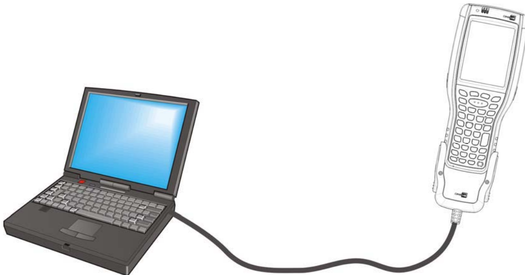
Figure 10: Direct Data Communication Using Snap-on Cable
