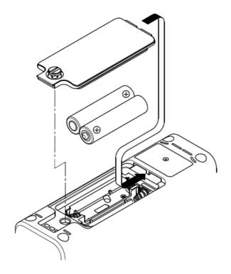
3. Replace the battery cover and tighten the screw securely.
