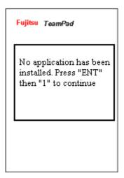
To begin the startup procedure: Hold down the ENT/SYS key, then press the "1" Key to Start the Touch panel calibration.
