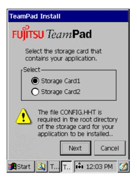
Select the Storage Card from which the software installation will occur. Select Storage Card1 if the application is to be loaded from a compact flash card located in the side of the unit. Select Storage Card2 if the application is to be loaded from a Type II flash card located in the top of the unit. For information regarding the CONFIG.HHT process, please refer to the "TeamPad 500 Programmer's Reference Guide".
