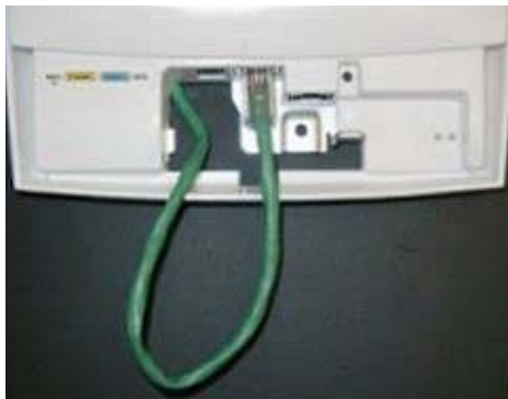
Figure 2-14 Looping the Ethernet Cable
