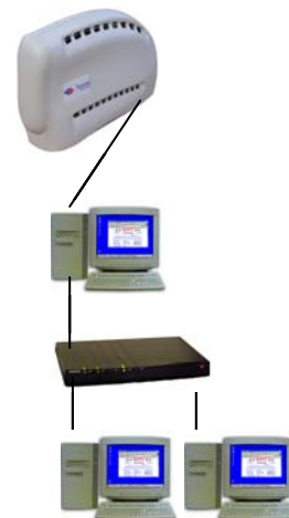
Modem connected to a PC, which is connected to a hub serving more than one PC
