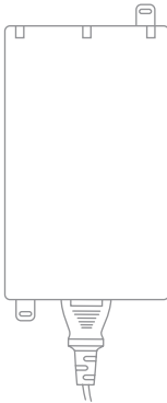
802.3af PoE power source (either PoE switch or Meraki 802.3af PoE Injector)
