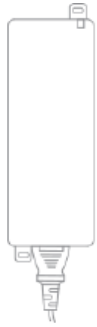
802.3at PoE power source (either PoE switch or Meraki 802.3at PoE Injector)
