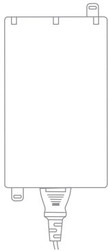
802.3at PoE power source (either PoE switch or Meraki 802.3at PoE Injector)
