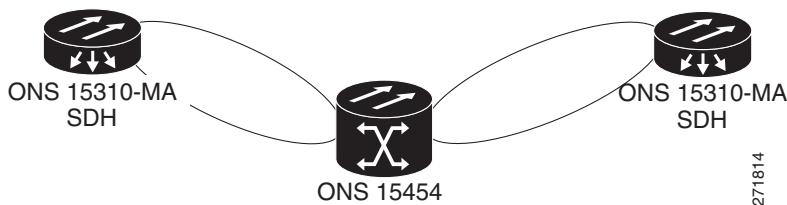
Figure 9-4 ONS 15454 SDH with Two ONS 15310-MA SDH Nodes Subtending Linear Multiplex Section Protection Configurations
