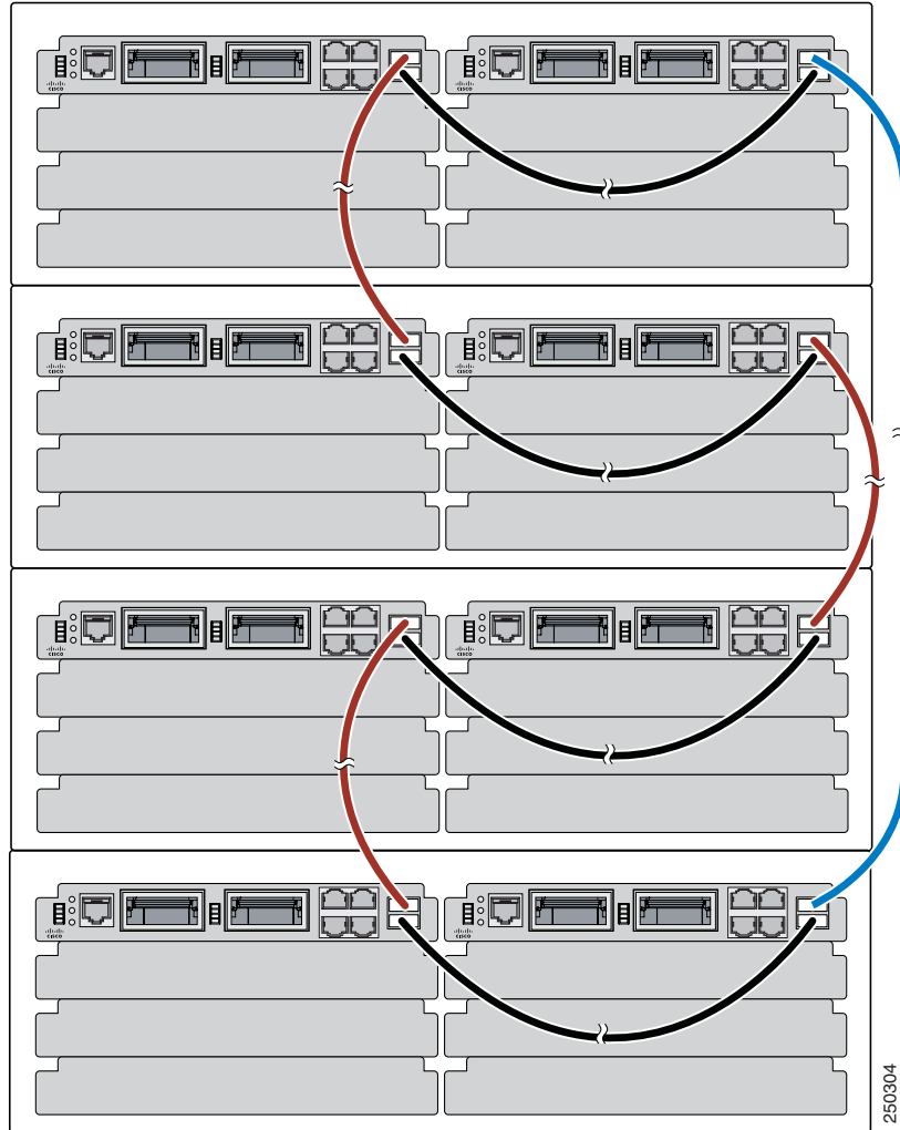
Figure 2-9 Stacking Eight Switch Modules in Four Blade Enclosures to Create One Stack
