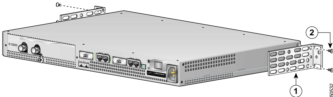
Figure 2-5 Attaching the Rack-Mount Brackets to the Rear of the Chassis
