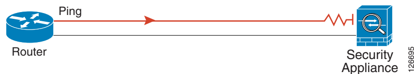
Figure 82-2 Ping Failure at the ASA Interface
