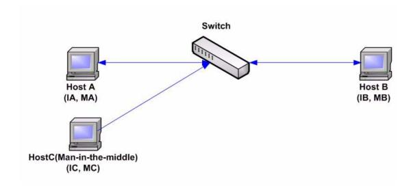
Hosts A, B, and C are connected to the switch on interfaces A, B and C, all of which are on the same subnet. Their IP, MAC addresses are shown in parentheses; for example, Host A uses IP address IA and MAC address MA. When Host A needs to communicate with Host B at the IP layer, it broadcasts an ARP request for the MAC address associated with IP address IB. Host B responds with an ARP reply. The switch and Host A update their ARP cache with the MAC and IP of Host B.
