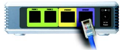
Figure 4-3: Connect to the Modem
