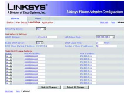
Figure 6-6: Router - LAN Setup Screen
