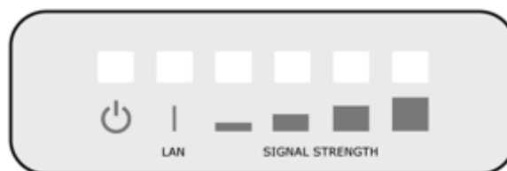
Fig. 3.3 - From Left To Right Status LEDs, Link/Boot LEDs
