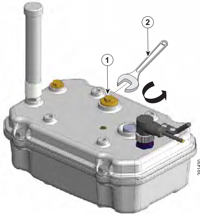
Figure 5-9 Removing the Console Port Cover
