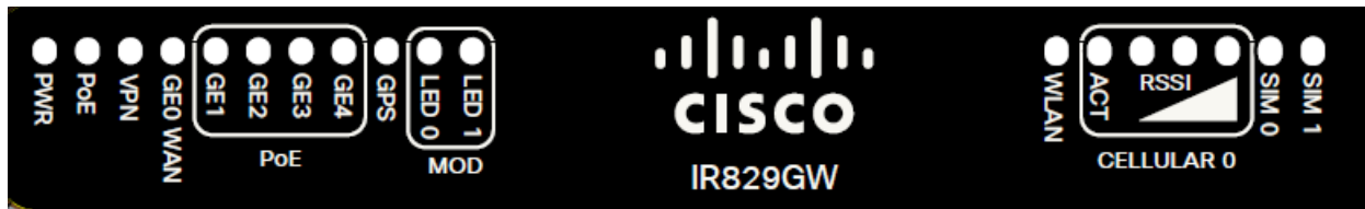
Figure 1-6 Cisco IR829 LED Detail
