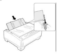
Adjust the head gap lever for the thickness of paper that you are using, then set the paper feed selector to friction mode position.
