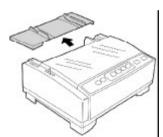
Adjust the head gap lever for the thickness of paper that you are using, then set the paper feed selector to the rear tractor mode position.
