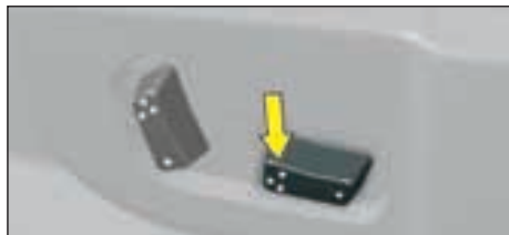
Seat cushion height and angle adjustment
