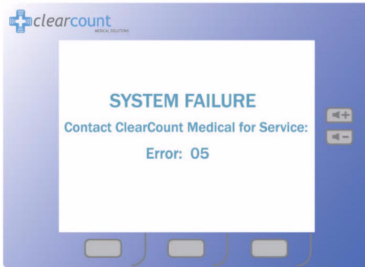
Figure 4-3 Example System Failure Screen
