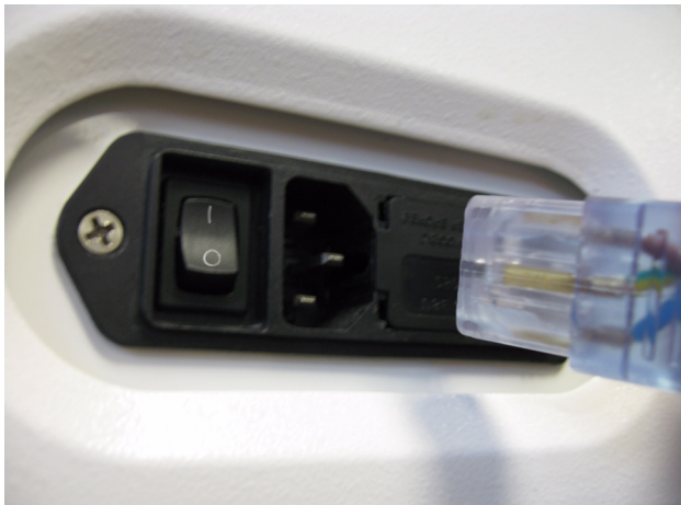
Figure 2-1 Location of On/Off Switch
