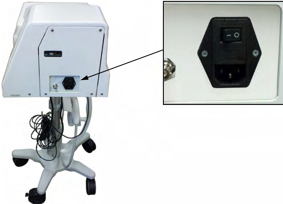
Figure 3-1 Location of On/Off Switch
