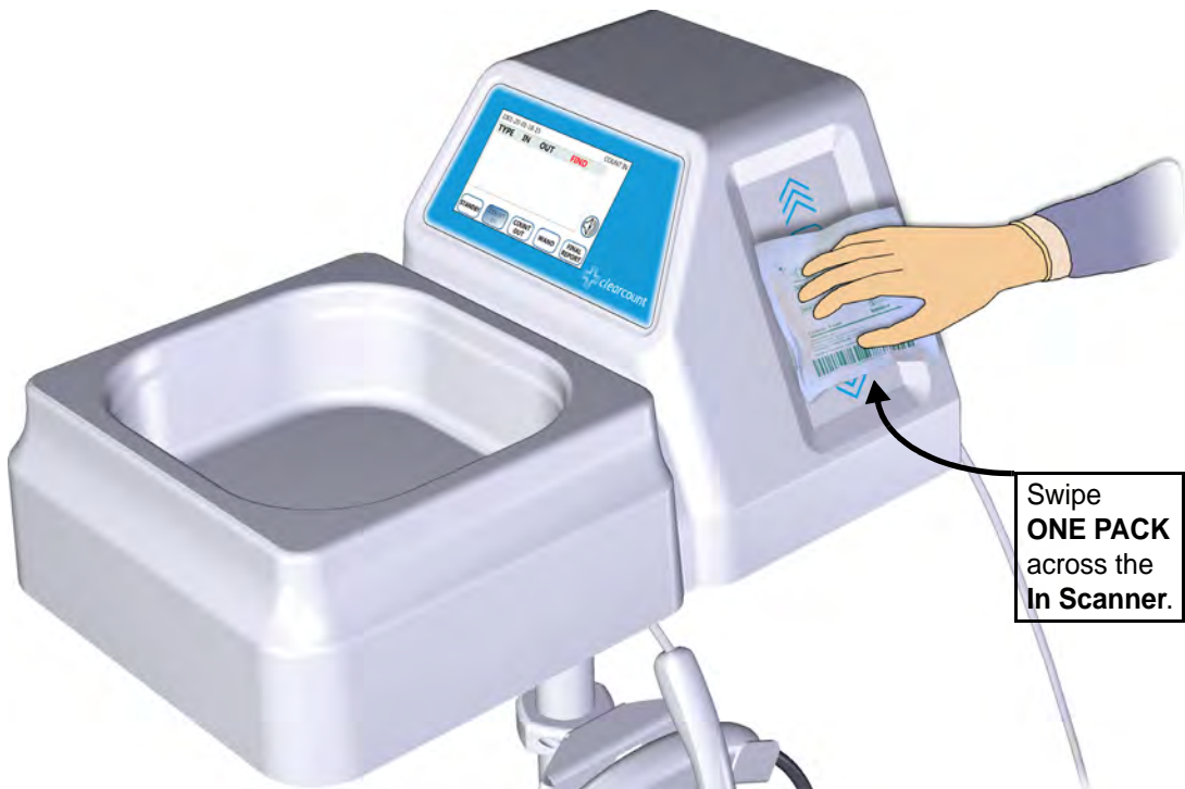
Figure 4-3 Scanning Sponge Packs Into the Surgical Case
