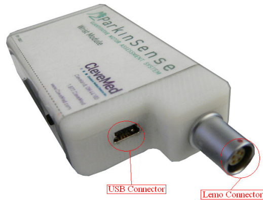
Figure 6. The ParkinSense wrist module includes both a mini USB and lemo connector.
