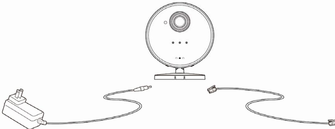
**Step 2.** Press and hold the **Privacy Button** and plug in the 5V DC power adapter.
