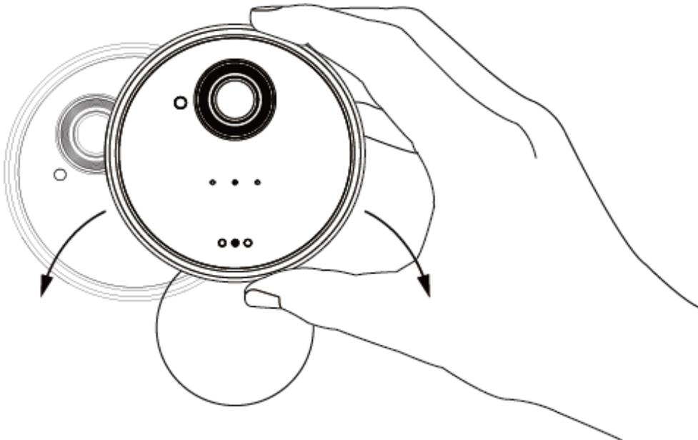
3. Rotate the camera stand base attached to the mounting base.
