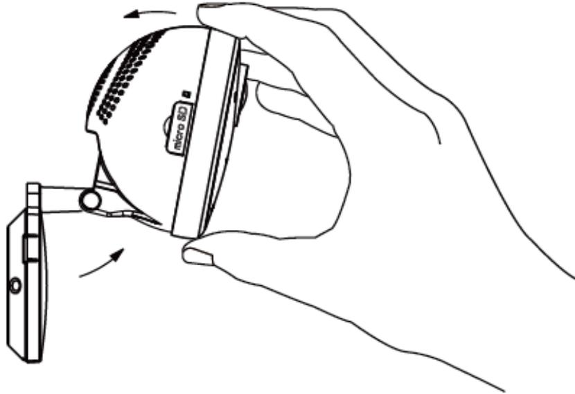
2. Rotate the camera clockwise or counterclockwise.
