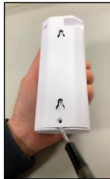
**Step 4:** Remove the old batteries and press the test button twice to fully discharge.
