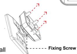
III. Screw the triangular bracket into the wall plugs with the two pointing sticks on bottom facing you.
