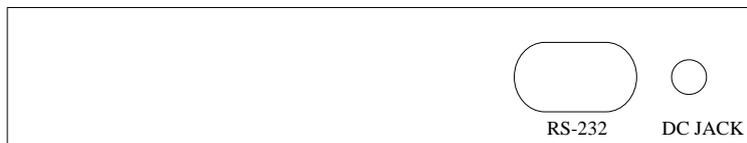
DC JACK: For connecting to 12V 500mA Power Adaptor
