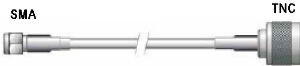
Picture 2-10 RF cable schematic chart
