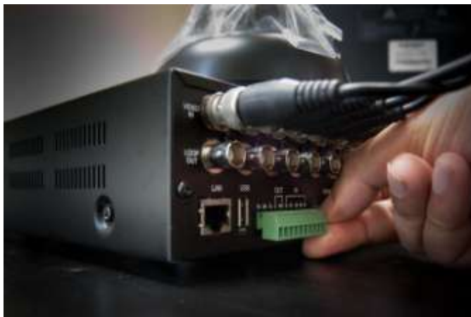
Figure 32 10-Way Terminal Block Connection
