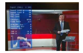
The displayed diagnostic data includes a spectrum display, signal to noise data, input power level and frequency. The received spectrum display is useful when checking for interference signals, the SNR indicated signal quality. For more information on use of this facility a domo training course is recommended.
