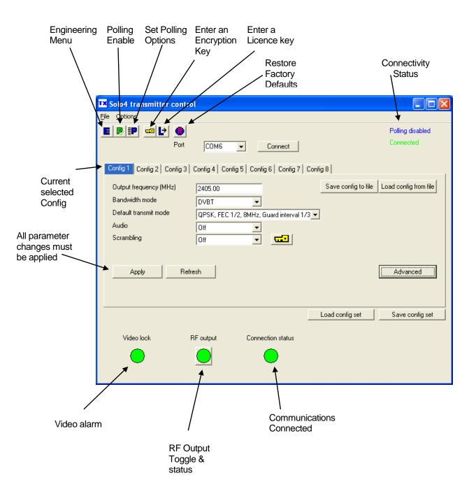
The 'Advanced' button allows the user to navigate to the controller page which exposes all available Transmitter settings.
