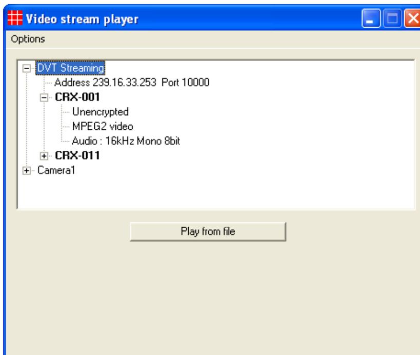
In this case we see that the service “CRX-001” is unencrypted, uses MPEG2 video encoding, and has single channel (mono) audio encoded with an 8-bit companding scheme with a sampling rate of 16kHz.
