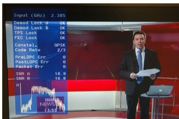
The displayed diagnostic data includes a spectrum display, signal to noise data, input power level and frequency. The received spectrum display is useful when checking for interference signals, the SNR indicated signal quality. For more information on use of this facility a demo training course is recommended and more information is available in section 13 of this manual.
